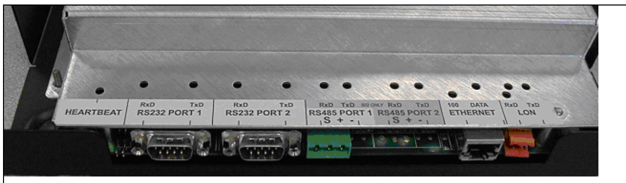
Figure 1 Connectors are located on the bottom edge of the JACE-5 controller.
